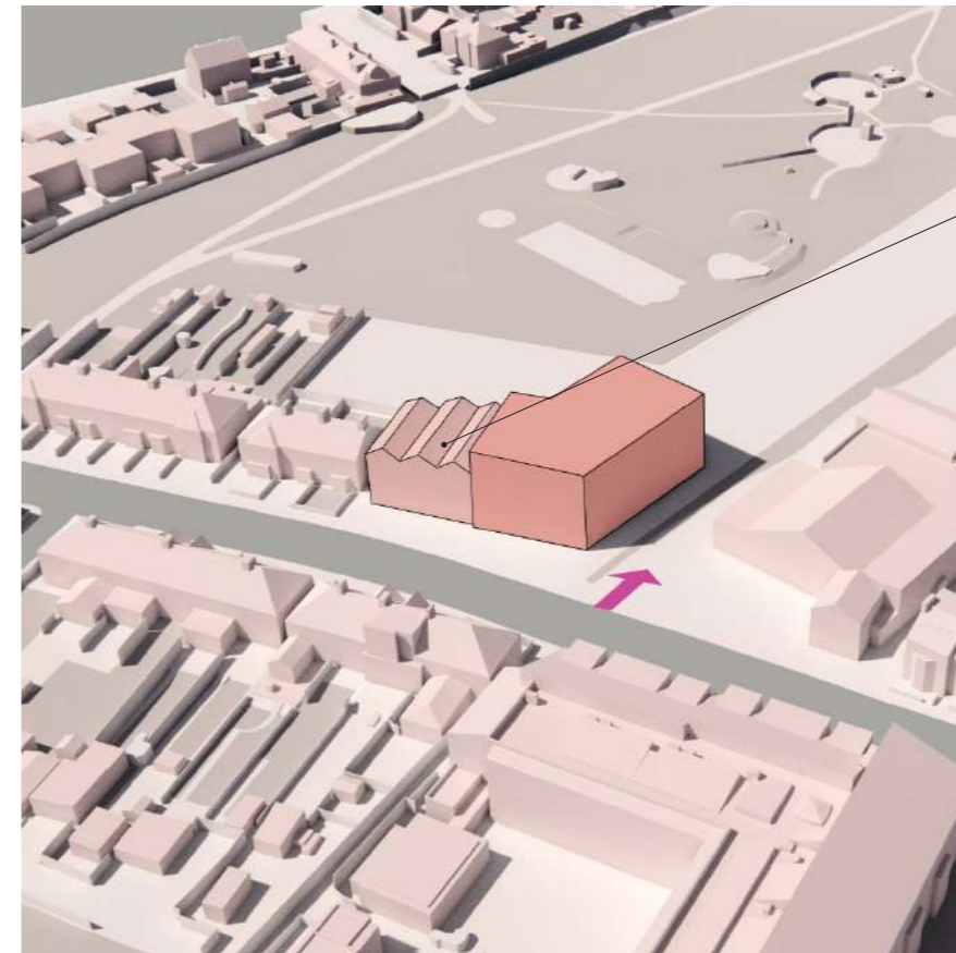
A pitched roof was added to further reduce the overall mass. The three-story section of the apartment also functions as a transitional element between the existing houses and the four-story part of the apartment building. The selection of roof types not only pays homage to the industrial heritage of the site but also provides insight into the architectural style of the proposed houses.
